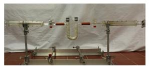
image: equipment to clean up the biogas. The U-pipe is filled with "Natronkalk".
