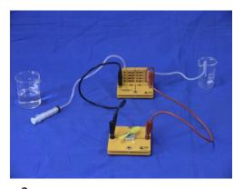
Installation of the fuel cell with voltage and ampere meter (see picture below)
